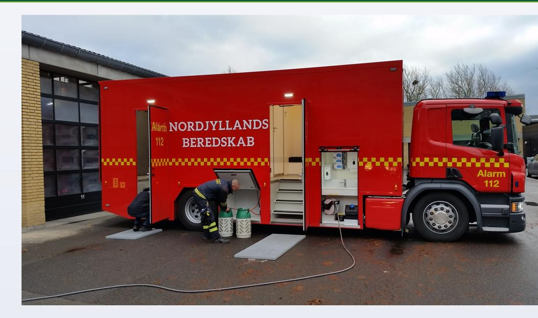
Truck drives to all fire scenes where the firefighters contaminated gear are bagged, sealed and handled. The firefighters are able to shower and change into clean dry clothes.
