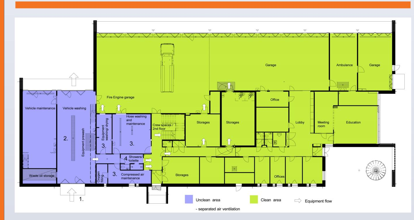
Clean fire station divided into clean/not clean areas to avoid cross contamination from contaminated equipment into living quarters. This station is build in Hollola, Finland.
